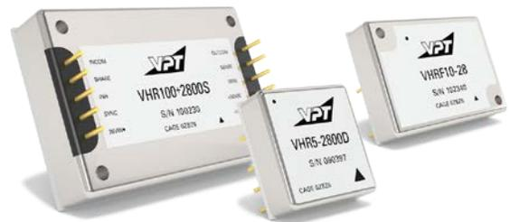
Designed to operate at full-load over a wide temperature range of -40°C to +100°C, the VHR Series also offers fixed frequency operation, soft-start, magnetic feedback, inhibit and current-limit protection. Additionally, the VHR Series includes companion EMI filters ranging from 1 to 20 amps.
