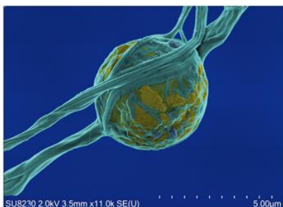
Algae spore trapped in spider silk coated with 5nm Au x 11k magnification
